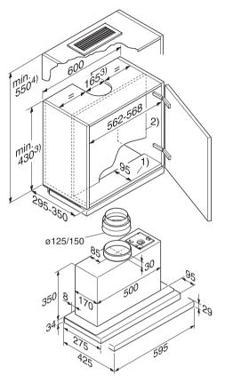
1) The front section of the wall housing unit must be fitted with a shelf to the depth of the partition wall. If the appliance is fitted further back, e.g. to accomodate a front panel, then the shelf depth should be correspondingly deeper.
